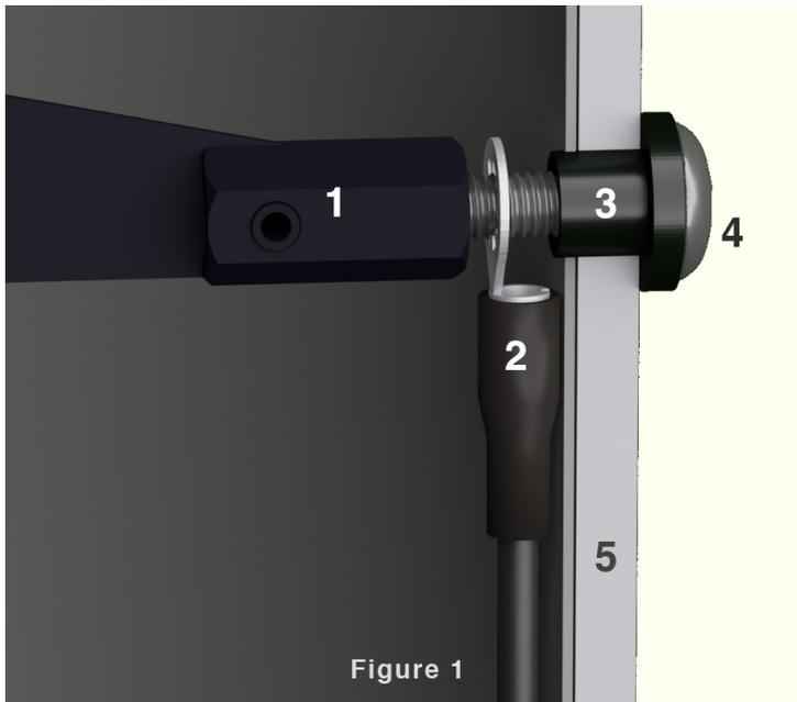
Figure 1 shows the recommended scheme for connecting power when installing into a metal tube, and illustrates how to use the insulation bushing (item 3). The bushing is not needed when installing into a non-conducting tube or cage material (wood, cardboard, fiberglass, plastic, etc.).
