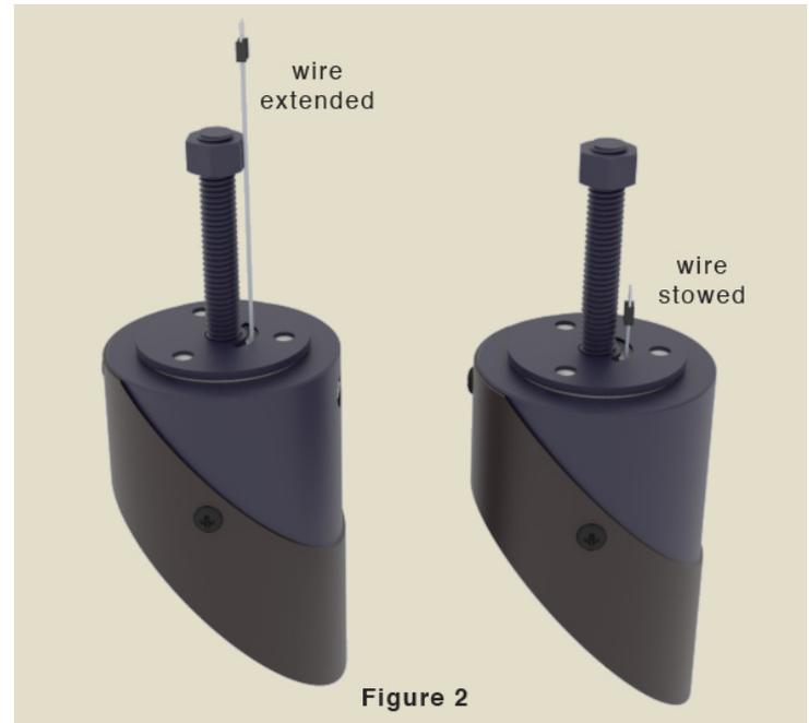
Fully extend the mirror holder's heater wire, and connect the micro-plug to the female plug on the spider (see Figure 2). The plug's polarity is not important. Push the wire into the holder body as you join the spider and holder.
